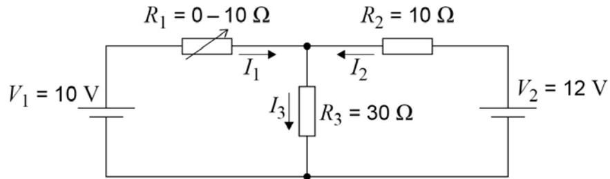
$R_1$  is a variable resistor with a resistance that varies between 0 and 10  $\Omega$ .
