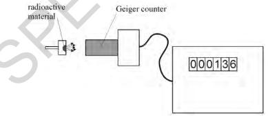
You place a thin sheet of paper between the source and the Geiger counter. You then replace the paper with a sheet of aluminium metal about 2 mm thick.
