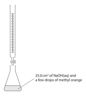
(a) Describe how to use the apparatus to find the volume of dilute sulfuric acid needed to neutralise the sodium hydroxide.
