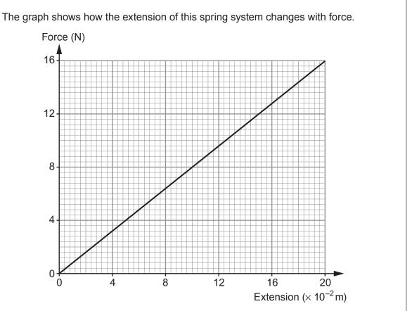
The two spring system is stretched and a model plastic plane of mass  $55 \times 10^{-3}$ kg is attached. A trigger is pressed, which releases one end of the spring system, and the plane is launched.
