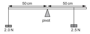
They hang a 2.0 N weight at one end, 50 cm from the pivot and another weight of 2.5 N somewhere on the other side of the pivot to make it balance.
