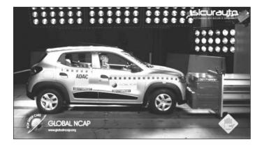
In one such test, a car of mass 1500kg travelling with an energy of 127500J strikes a solid barrier and stops. The force applied to the car by the barrier is 500000N.
