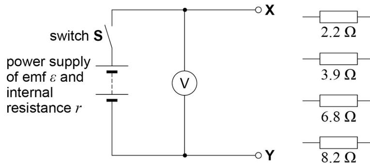
The student can change the external resistance  $R$  of the circuit between terminals  $X$  and  $Y$ . This is done by connecting different combinations of **two** resistors in series or in parallel between  $X$  and  $Y$ . This method can produce **12 different values** for  $R$ .
