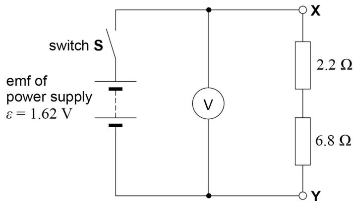
When **S** is closed the voltmeter reading  $V$  is 1.14 V.
