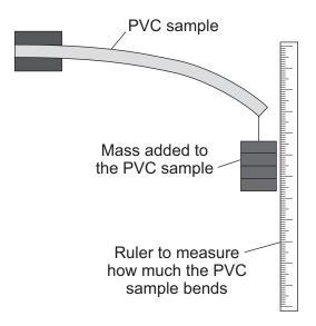
He measured the bending of PVC samples containing different percentages of an added chemical called a plasticiser. The PVC samples were all the same size.
