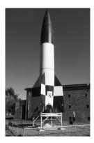
V2 rockets were powered by liquid oxygen and ethanol. Oxygen and ethanol react to produce carbon dioxide and water.
