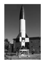
V2 rockets were powered by liquid oxygen and ethanol. Oxygen and ethanol react to produce carbon dioxide and water.
