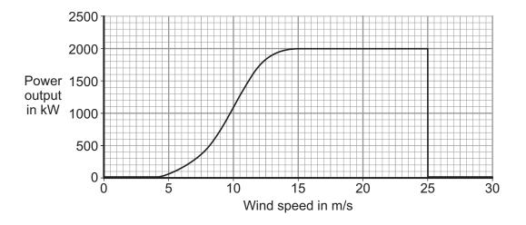
The turbine is designed to operate best at a minimum wind speed of 15 m/s. This is called the rated wind speed.
