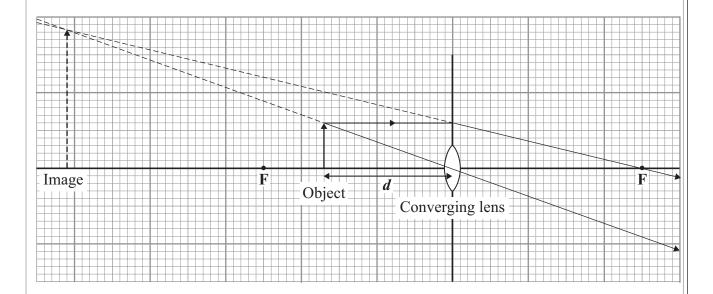
**8** (a) (i) The height of the object and the height of its image are drawn to scale.
