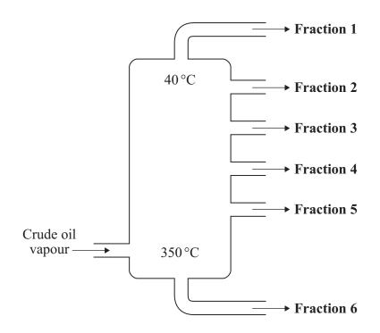
6A Crude oil vapour enters the fractionating column.
